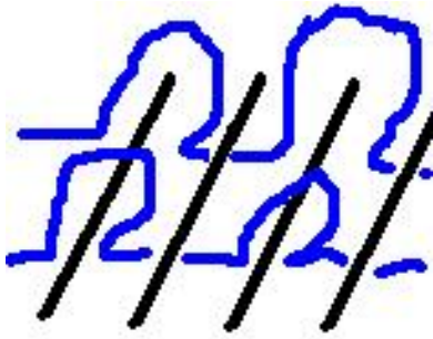
Figure 3: A yarn loop is actually a segment of warp thread
