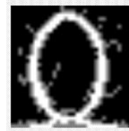
Figure 10: A typical yarn loop volume layer. Defined by a 32 \times 32 pixel image.
